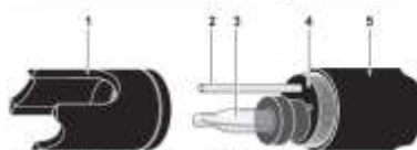
Fig. 1.7 Structure of the SensoLyt 650-7 pH/ORP armature
